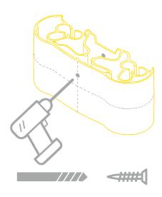
DRILL A HOLE THROUGH THE FRONT AND BACK WALLS OF THE GUARD
